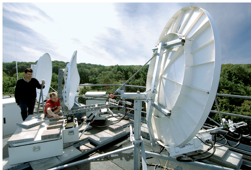
Figure 4: Bernd Blanzano (Technical University Graz, on the left) and Jürgen Becker (PTB) adjust the antenna of the portable TWSTFT ground station of TU Graz during the latest link calibration campaign in September 2008. The other antennae belong to PTB reference stations.
