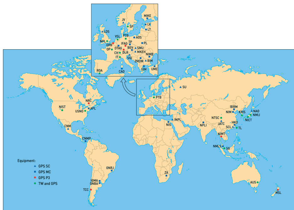
Figure 3: Geographical distribution of the laboratories that contribute to TAI and employed clock comparison methods [17]. Adapted with kind permission of BIPM.
